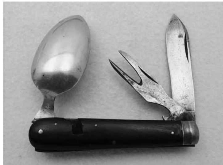
Ulster Knife Co - This slip apart knife has three functions in the one blade. It is a two tine fork, a can opener and a crown cap opener. A little trivia is that the invention of the crown cap was 1891, and the Ulster name started in 1876.
