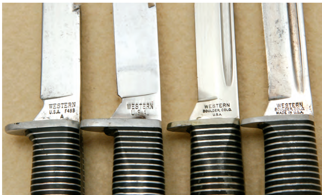
A variety of different tang stamps found on Black Beauty knives from the late 1950s through the early 1980s.
