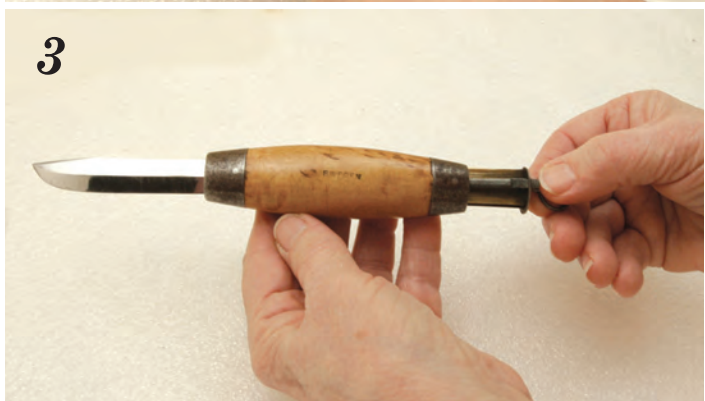
(1) The opening of this knife is easy and safe. While the latch is depressed, the thumb is used to push the inner knife assembly out of the barrel. (2) When the inner frame clears the barrel, the barrel itself fulcrums the knife into the open position. (3) Pushing the knife blade forward until the latch engages makes the knife ready for use. (4) Similarly to #2, the barrel can be used to close the blade without touching it when the task is completed. (5) Typical Swedish barrel knife with the inner brass frame fully removed from the barrel handle.
