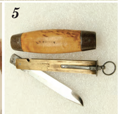
(1) The opening of this knife is easy and safe. While the latch is depressed, the thumb is used to push the inner knife assembly out of the barrel. (2) When the inner frame clears the barrel, the barrel itself fulcrums the knife into the open position. (3) Pushing the knife blade forward until the latch engages makes the knife ready for use. (4) Similarly to #2, the barrel can be used to close the blade without touching it when the task is completed. (5) Typical Swedish barrel knife with the inner brass frame fully removed from the barrel handle.
