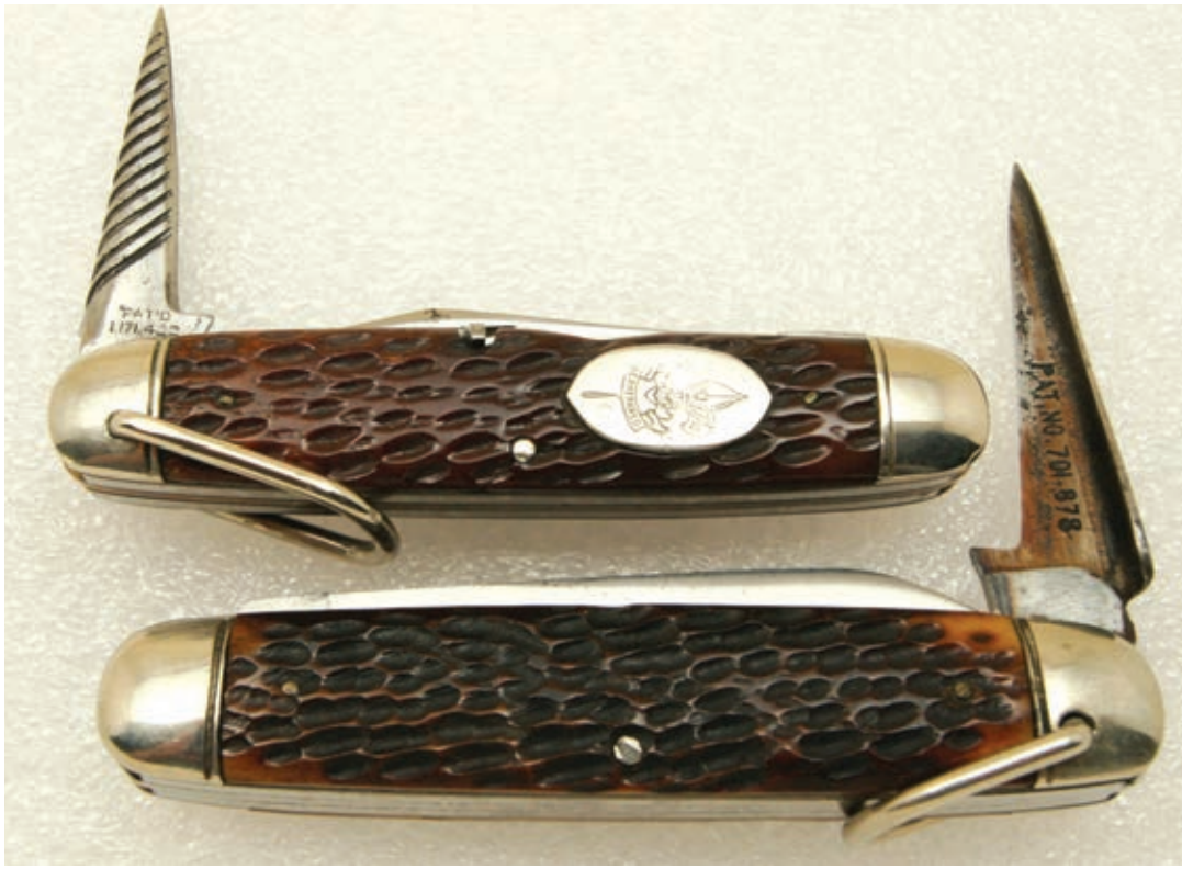
The spiral design punch was first patented in 1916 and was used exclusively by the New York Knife Company. The spiral idea was first introduced by the NYKCO and was copied by several other manufacturers after the patent expired.
