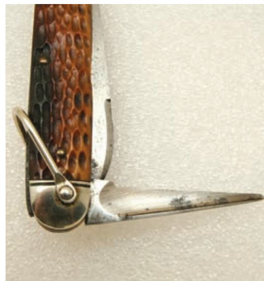
Stout, strong and a simple design typify the Schrade Cutlery Co. punch blade. The vertical grind lines that end near the tang provide clues to identify punch blades made by this company. This is an oval shape left by the grind.
