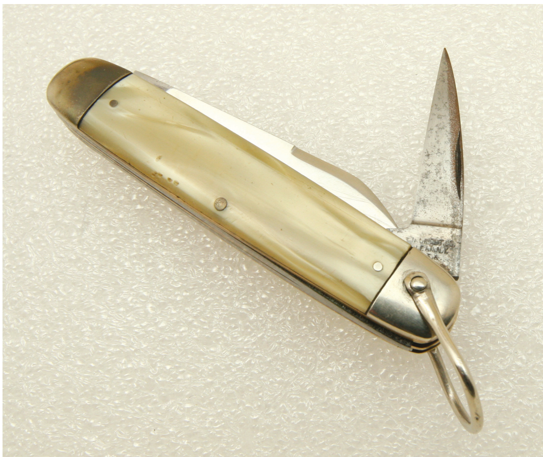
The utility pattern knife put out by Union in the 1920s era had light yellow celluloid handles. Over time they started to off-gas a nitric acid by product and, as a result, rusted any metal surface exposed. There are many reasons for this, but that is a paper unto itself. The pictured knife shows the ravages of this deterioration on the upper edge of the punch blade and on the bolster.
