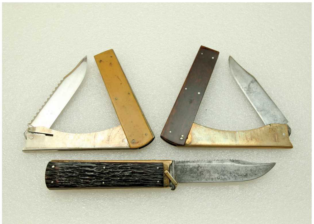
Fishing knives seem to be a Union/KA-BAR specialty. Marble's came out with the first fishing tri-fold knife in the early 1910 era. The tri-fold was touted as a safety knife and was a fun knife to operate. A patent was granted in 1924 (#1,486,725) which incorporated a latching device for the tri-fold. They also introduced the liner lock on this knife to provide rigidity when the knife was opened. This was an early use of a liner lock on a knife.
