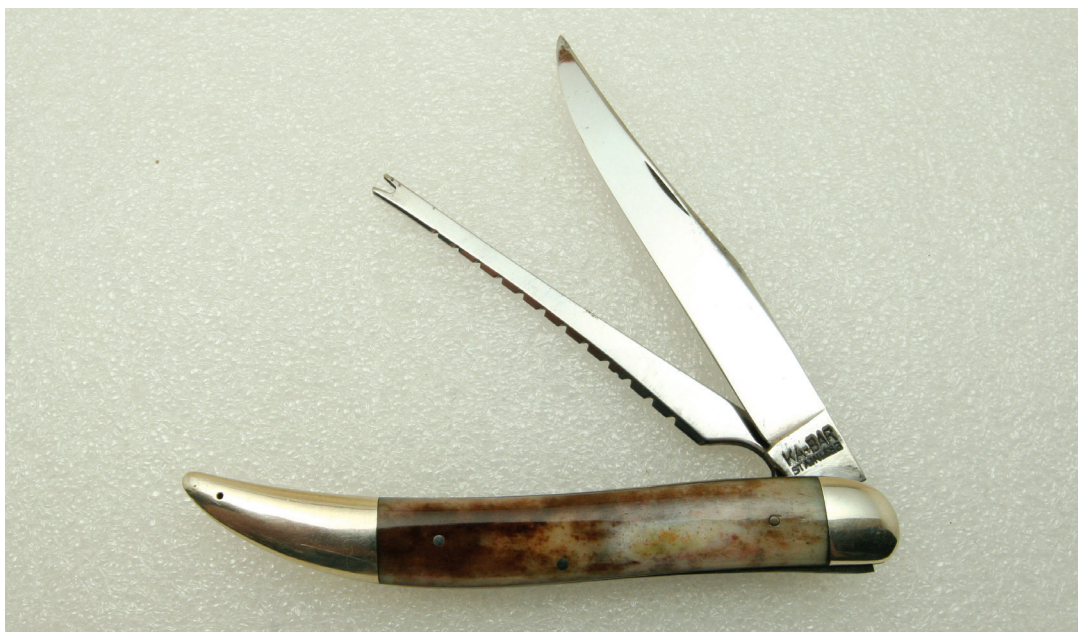
My father was an addictive fisherman who had this knife in his fishing box for years. It is patented #1,788,656 (1/13/1931) and had those destructive yellow celluloid handles. My inheritance. I had Michael Yoh restore the handles with smooth bone handles. The stainless was impervious to the celluloid gassing, so I now have a fantastic looking KA-BAR fish knife to pass down to my fishing-less family.
