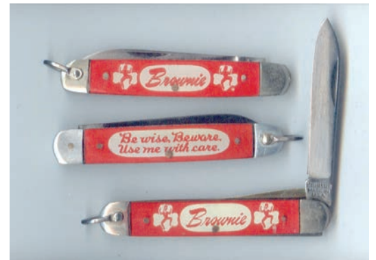
These 1950s vintage Brownie knives by Kutmaster have experienced off-gassing and handle shrinkage. It is possible they have been exposed to an environmental trigger that has prompted their decomposition. The open knife shows heavy staining on the exposed part of the blade when it is closed. The “Be Wise, Beware” has a double meaning here.
