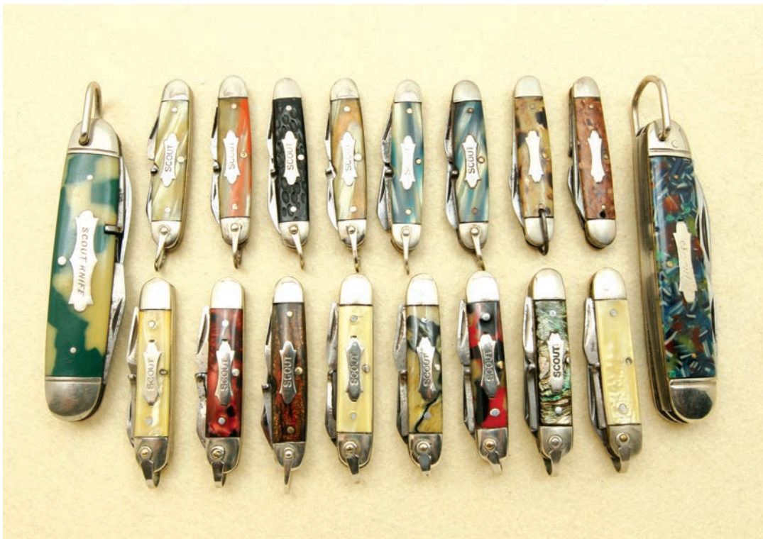
These 2½” punch board or carnival knives of the 1920s-1930s show no signs of deterioration. The binding added to the celluloid and good storage can explain why they are stable today.
