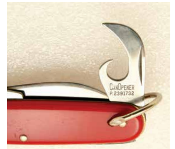
The Imperial safety can opener was the device that could safely "open a can of worms." The patent number is proudly stamped on the blade, as is the description, should anyone not know this device's purpose.
