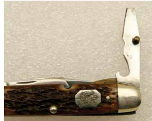
The Cattaraugus Whitt-L-Kraft knife has a can opener that is often overlooked. The scraper edge used in wood carving can also be used to open a can. By allowing the pin to ride on the edge of the can, the can opens easily.
