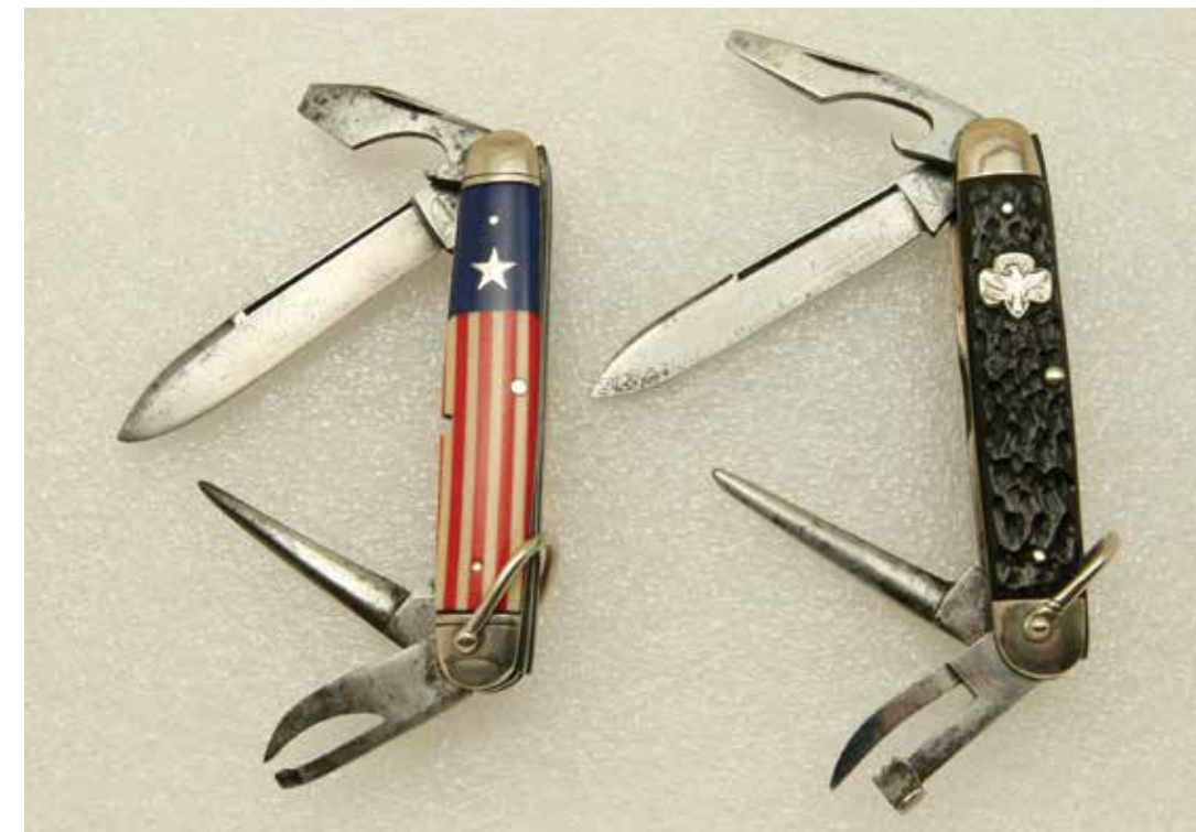
Remington used the popular "D" (Style 1) can opener in this Red White and Blue Patriotic Knife (left). After 1924 a patented two-piece can opener was used as shown in this Girl Scout utility knife (right).
