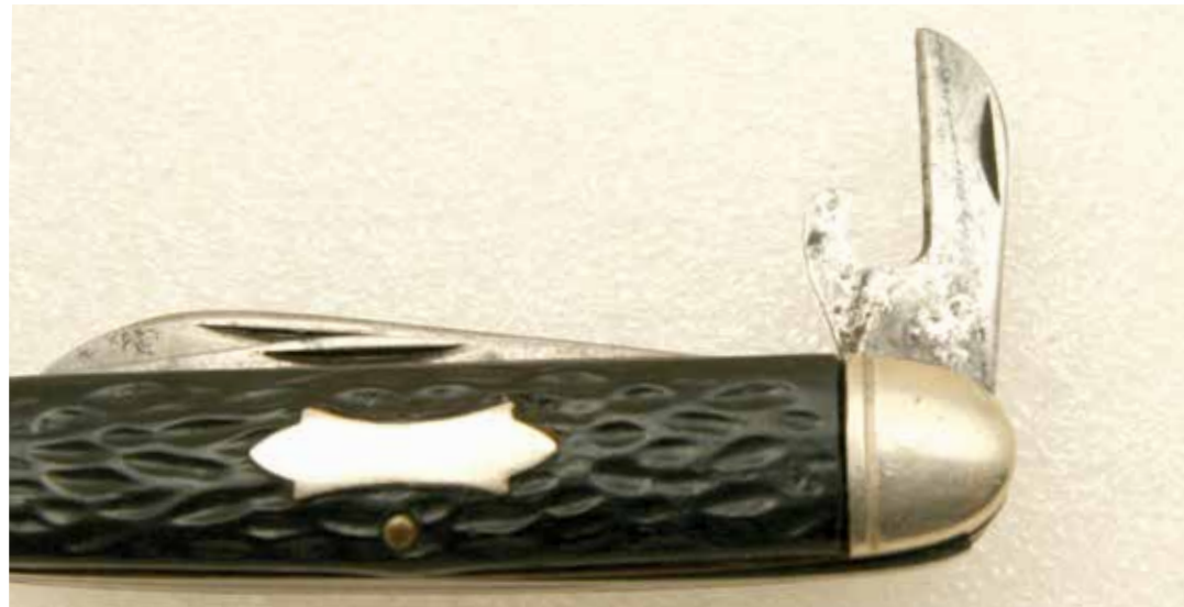
This four line Camillus can opener dates to the 1940s as a work around the Imperial patented safety device. It is pretty close to the safety design, but uses a two piece construction. This style can also be found on 1950s Boker knives.
