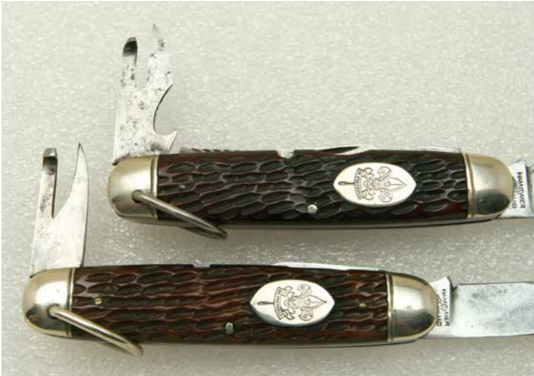
The classic style Broken D (Style 1) can opener was used by New York Knife Company (NYKCO) in two configurations. Note the cap lifter combination and also the broken shotshell extractor tab.
