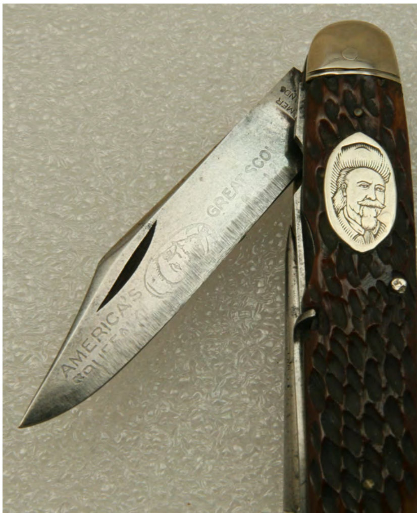
This view shows the etch on the main clip point blade as well as the portrait shield of Buffalo Bill. Lined bolsters usually suggest a top line quality knife.
