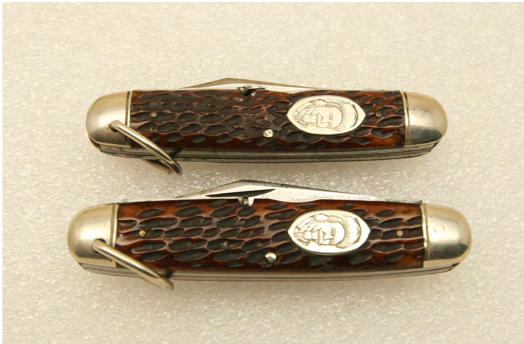
The Buffalo Bill knives were offered in two sizes. One was the standard utility size, and the other was the junior size; both had clip point blades. The regular BSA Official Knives had a spear point main blade.
