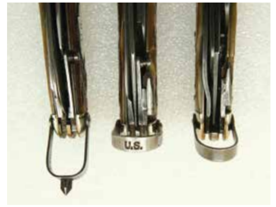
During WWII Ulster made knives specifically for the mountain U.S. Ski Patrols. At one point Phillips head screws were used on the ski bindings. This called for a five blade pocket tool with a Phillips driver for unexpected repair. The first design had this tool on the bail. Later designs incorporated the driver in the frame. Later bails had a hefty U.S. marked bail and then a bail that was unmarked.
